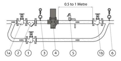
Isolation Valves - 1, 1a & 1b / Filter - 2 / Manometer and Gauge - 3, 6 Reducing Valve - 4 / Safety Valve - 5
